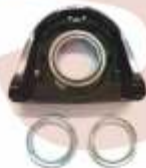
YSM VOL 42 VOLVO CENTRE BEARING DIA=100 X 13 MM OEM NO. 81394106018
