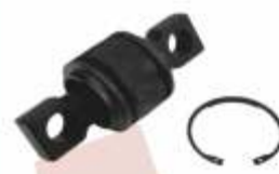
YSM SC 3 SCANIA REP. KIT, LINK OD-75, L-148, B-19, BD-115 THICKNESS-24 OEM NO. 2096392/1722753
