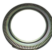
YSM 238 BPW RINGS ABS 100 SLOTS SIZE-105/156x21.7 OEM NO. 0531007301
