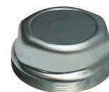
YSM 187 BPW HUB CAP 6.5-9 TONS (M115 X 2) OEM NO. 0321223090
