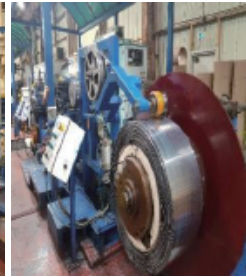
Traverse Winding Line
