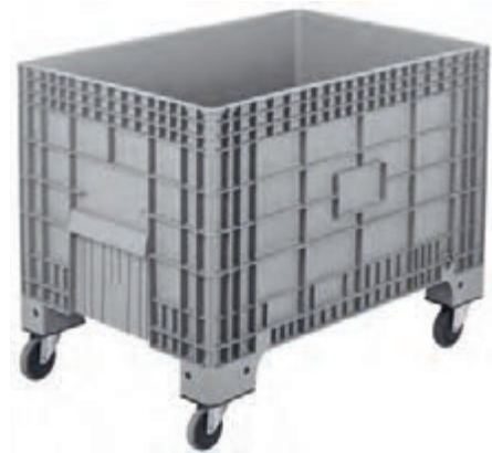
K-550 T En/W Boy/L Yük/H Hacim Dynamic Static Dış / Ext 800 x 1200 x 925 mm Volume Capacity Capacity İç / Int 732 x 1108 x 617 mm 500 Lt 400 Kg 2500 Kg Kapalı / Closed Ağırlık / Weight 25,50 kg
