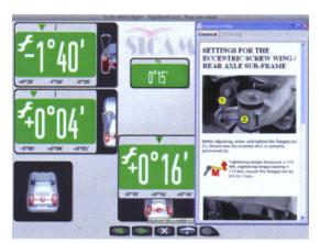
Graphic illustration guide the operator during the adjustment phase
