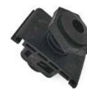
HOOD MOULDING Front, hood adjustment screw, original.
