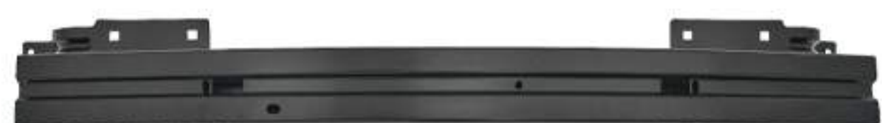
BUMPER REINFORCEMENT Upper, plastic.
