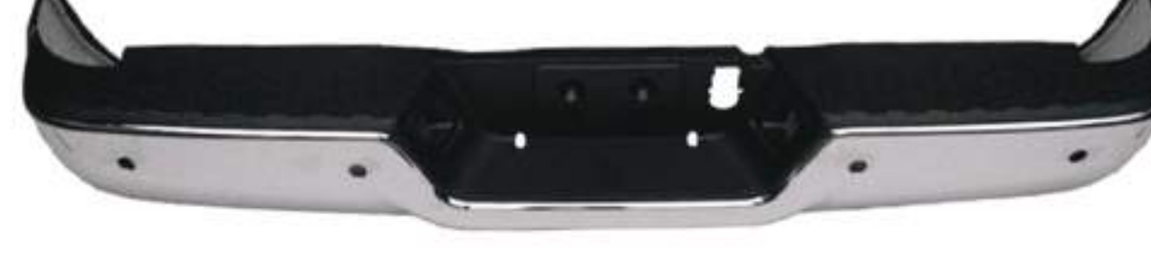
BUMPER REAR R2500, R3500, (- 15), with parktronics' holes, with space for 1 muffler, chrome. PDG40127BA
