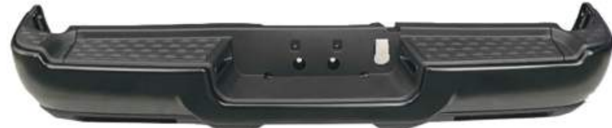
BUMPER REAR R2500, R3500, with 6 holes for parktronic, with bumper lining, to be painted, with hole for foglamp. PDG40190BA
