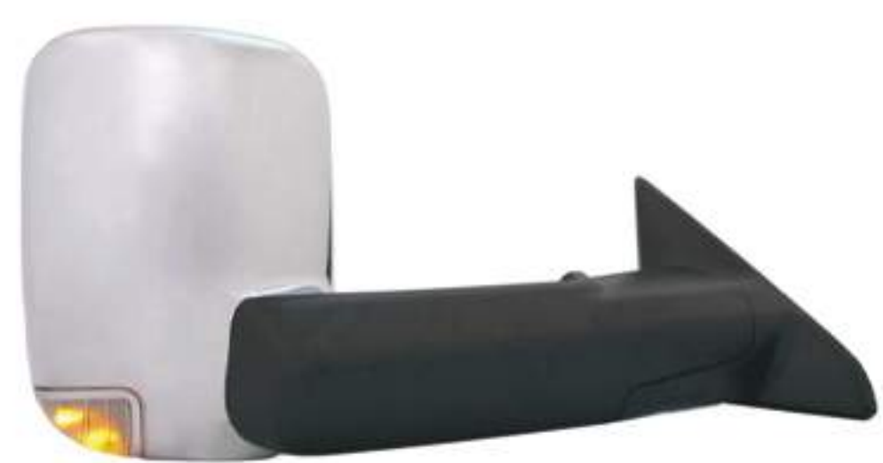
MIRROR Electric, heated, with memory, with legs lighting, with indicator.
