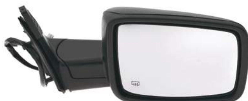
MIRROR (- 15), electric, heated, chromed glass, 5 contacts, 8 wires, with legs lighting, with indicator.
