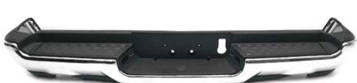
BUMPER REAR R1500, without hole for parktronics, with 2 holes for muffler exhaust pipe, chrome.
