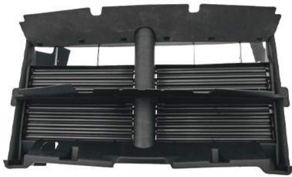
AIR INTAKE 3.6L, 5.7L, R1500, without motor.
