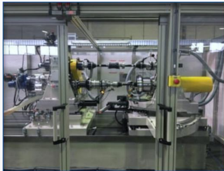
NVH test rig(Germany)
