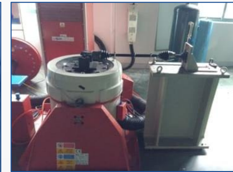
Natural frequency measurement rig (Germany)
