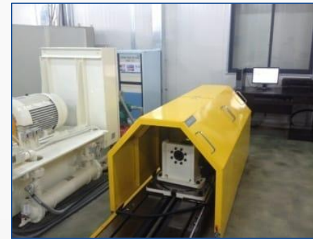
Torsional fatigue test rig (Japan)
