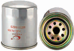
FX0-XF-003 Largest OD: 80(mm) Overall Height: 100(mm) Thread Size: M20X1.5 OEM: ME016823 MITSUBISHI: 055923570, ME016823 BF825F
