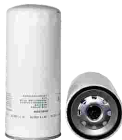
FXO-B0-006 Largest OD: 108(mm) Overall Height: 260(mm) Thread Size: 1,1/8"-16 OEM: W11102/16 MANN: W11102/16
