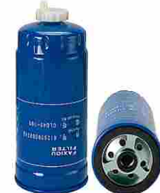
FXO-AHF-004 Largest OD: 84(mm) Overall Height: 186(mm) Thread Size: M16×1.5
