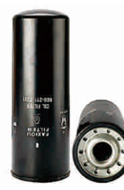
FXO-FO-011 Largest OD: 108(mm) Overall Height: (270mm) Thread Size: 1 1/2"-12
