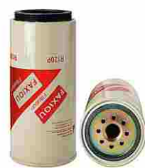
FXO-HF-009 Largest OD: 108(mm) Overall Height: 218(mm) Thread Size: 1"-14UNF
