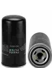
FXO-B0-009 Largest OD: 94(mm) Overall Height: 170(mm) Thread Size: 1"-12UNF OEM: WD950/2 MANN: WD950/2 HENGST: H19WD02
