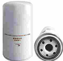
FXO-BL-004 Largest OD: 93(mm) Overall Height: 175(mm) Thread Size: M27X2
