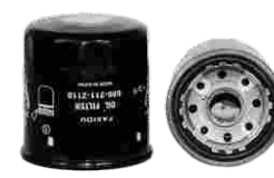
FXO-FO-001 Largest OD: 74(mm) Overall Height: 80(mm) Thread Size: 3/4"-16
