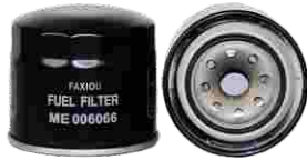
FX0-XF-001 Largest OD: 89(mm) Overall Height: 81(mm) Thread Size: M20X1.5 OEM: ME006066 MANN: WK818/80 CAT: 094-7073
