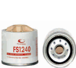
FXO-DF-025 Largest OD: 94(mm) Overall Height: 90(mm) Thread Size: 1"-14UNF OEM: FS1240 FLEETGUARD: FS1240
