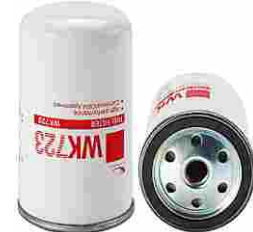
FXO-BF-0011 Largest OD: 77(mm) Overall Height: 122(mm) Thread Size: M16X1.5 OEM: Wk723 CAT: 5W-3394 DEUTZ: 01180597 VOLVO: 11706667 RENAULT: 5000814227 STEYR: 2203710/0 HENGST: H60WK03
