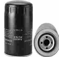
FXO-B0-014 Largest OD: 108(mm) Overall Height: 180(mm) Thread Size: 1"-12UNF OEM: W1168/5 MANN: W1168/5 003 184 33 01
