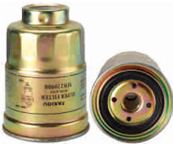
FX0-XF-009 Largest OD: 92(mm) Overall Height: 133(mm) Thread Size: M20X1.5 OEM: MB220900 MITSUBISHI: MB220900 HYUNDAI: 31973-44000 MAZDA: 1456-23570A SUZUKI: 15410-78E01
