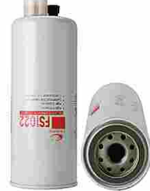
FXO-DF-033 Largest OD: 94(mm) Overall Height: 238.5(mm) Thread Size: 1"-14UNF OEM: FS1022 FLEETGUARD: FS1022
