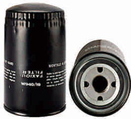
FXO-B0-003 Largest OD: 94(mm) Overall Height: 142(mm) Thread Size: 1"-12UNF OEM: W940/18 MANN: W940/18 HENGST: H17W04 DEUTZ: 01173481 VOLVO: 11700375 FAWDE: 1012010-29D
