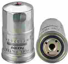
FX0-XF-004 Largest OD: 90(mm) Overall Height: 142(mm) Thread Size: M20X1.5 OEM: ME132526 MITSUBISHI: ME132526 MANN: WK940/37X PURFLUX: CS766 HENGST: H237WK
