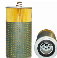
FXO-B0-022 Largest OD:120 (mm) Overall Height: 274(mm) Thread Size: Φ 56, Φ 14 OEM: H12110/2X MANN: H12110/2X HENGST: E251HD11 RENAULT: 5000043298
