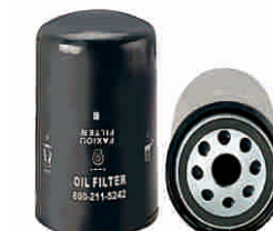
FXO-FO-004 Largest OD: 94(mm) Overall Height: 154(mm) Thread Size: 1"-12
