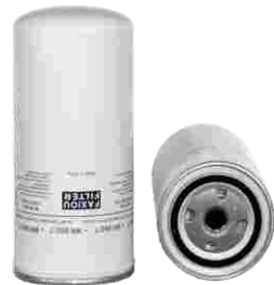
FXO-BF-003 Largest OD: 94(mm) Overall Height: 215(mm) Thread Size: M18×1.5 OEM: WK962/7 MANN: WK962/7 VOLVO: 8193841 VG1560080012
