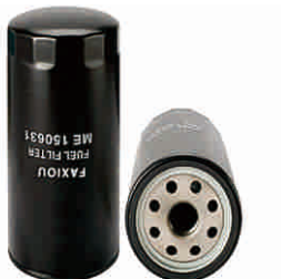
FX0-XF-006 Largest OD: 108(mm) Overall Height: 200(mm) Thread Size: 1 1/8"-16 OEM: ME150631
