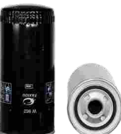
FXO-B0-012 Largest OD: 94(mm) Overall Height: 208(mm) Thread Size: 1"-12UNF OEM: W962MANN: W962 HENGST: H18W01 IVECO: 1160025 BENZ: 0011849601 RENAULT: 0024164103 VOLVO: 11993545-0 DEUTZ: 01174421
