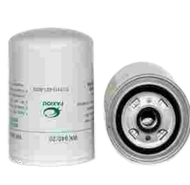
FXO-BF-002 Largest OD: 94(mm) Overall Height: 145 (mm) Thread Size: M18X1.5 OEM: WK940/20 MANN: WK940/20 CNHTC: VG1540080310 FAWDE: 1117011-621-0000
