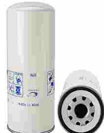
FXO-BF-004 Largest OD: 108(mm) Overall Height: 260(mm) Thread Size: M32X1.5 OEM: WDK11102/4 MANN: WDK11102/4
