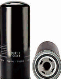
FXO-B0-011 Largest OD: 94(mm) Overall Height: 214(mm) Thread Size: 1"-12UNF OEM: Wd962 MANN: W0962 HENGST: H18W001 DEUTZ: 01180977 KOMATSU: PZF848101162 RENAULT: 5000289323 VOLVO: 4720309
