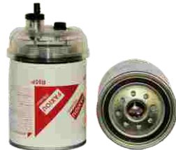
FXO-HF-002 Largest OD: 108(mm) Overall Height: 195(mm) Thread Size: 1"-14UNF
