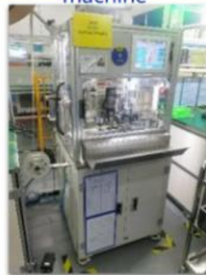
Automatic threading and crimping terminal all-in-one machine
