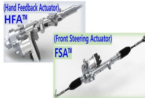
Redundant By-Wire-EPS, for light/mid-duty vehicles, with Road Force Feedback
