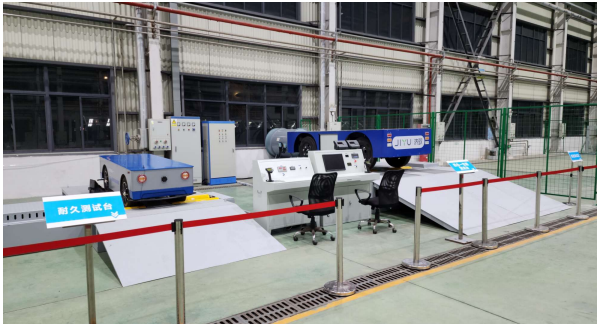
Chassis-By-Wire durability dynamometer & performance test dynamometer.
