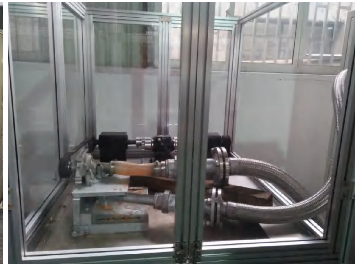
水泵可靠性测试台 INTERNAL COMBUSTION ENGINE COOLING PUMPS RELIABILITY TEST-BED
