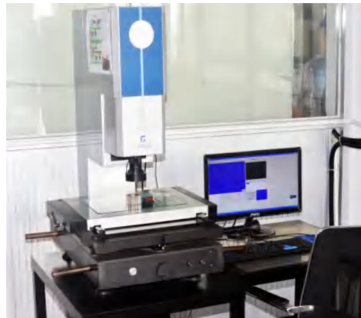
影像仪 VIDEO MEASUREMENT INSTRUMENT
