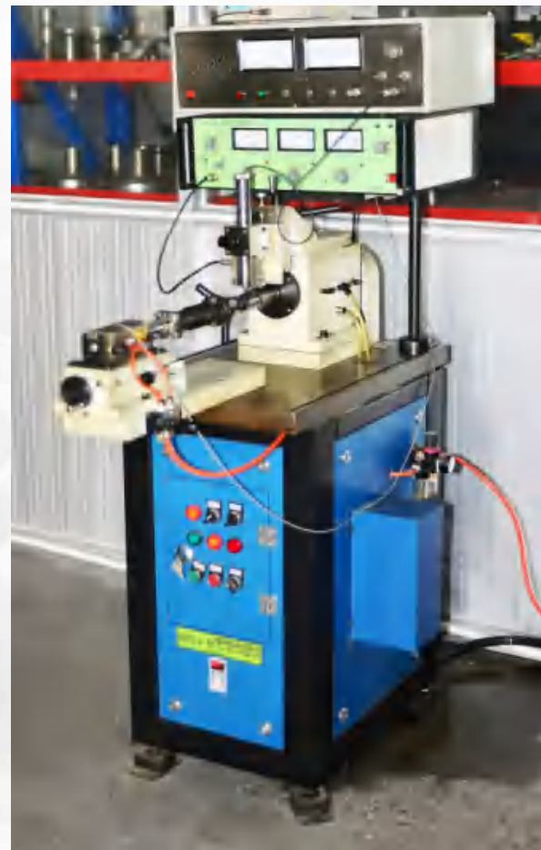
轴承振动测量仪 BEARING VIBRATION MEASUREMENT INSTRUMENT
