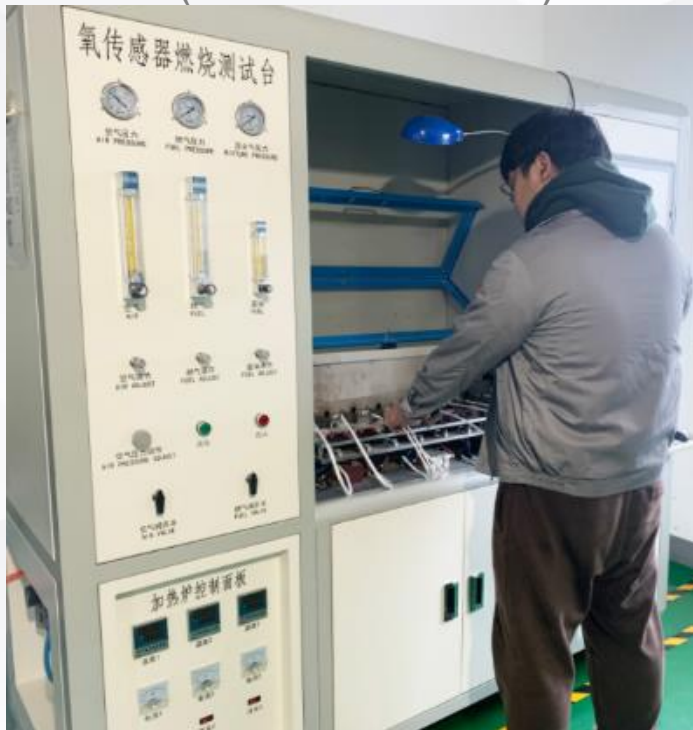
燃烧测试台 (Combustion test)
