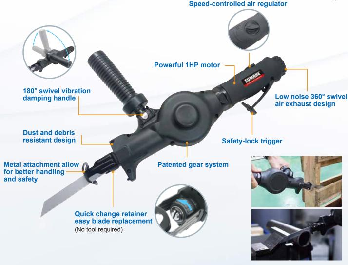
**ST-BW710** 2,400 spm Suitable for METAL cutting
