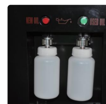
Oil injection & drain controlled by switch
