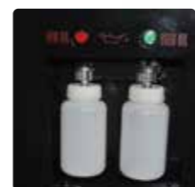
Oil injection & drain controlled by switch
