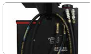
Oil injection & drain Controlled by switch
