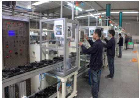
Korean Automatic Rotor assembly Line
