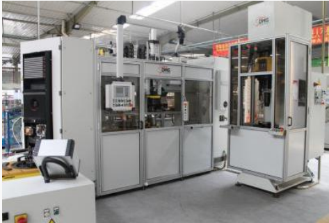
Italian DMG automatic stator wire winding machine
