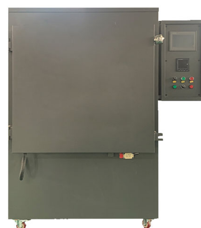
BG No.:502004 Intelligent DPF/SCR High temperature regeneration furnace
