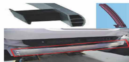
前后防撞梁 Front and rear anti-collision beams
