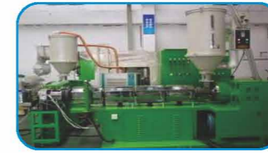
TPV Extrusion machine Quantity: 3 units Realize the function : The 4 materials are extruded together
