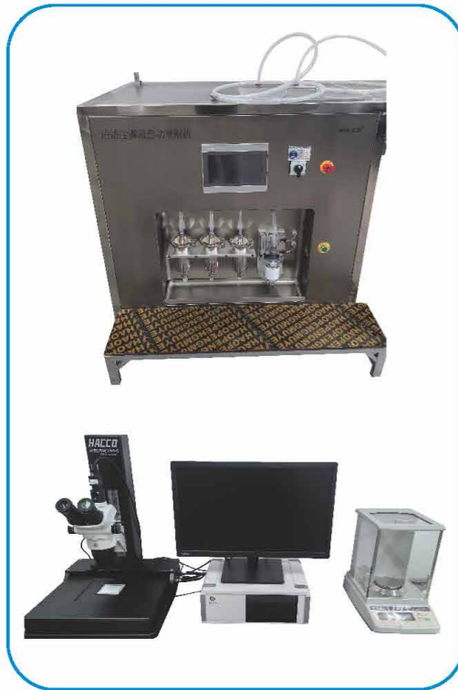
清洁度检测系统 Cleanliness inspection system
