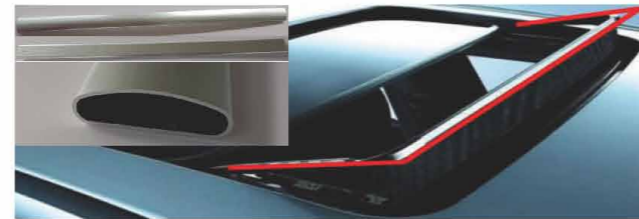
天窗挡风金属杆、导风板 Skylight air baffle metal pole and air deflector
