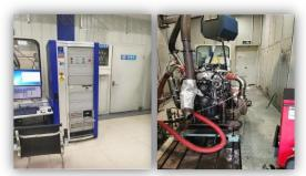
AVL gas analyzer & engine bench test
