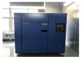
thermal shock test chamber
