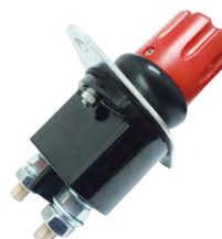
E061026 Push off in emergency Silver plated copper studs Max. 250A continuous
