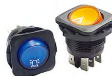
E067447 On-On 6P DPDT, 12VDC 20A Mounting: Ø20.2mm Option: Printed symbol
