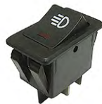
E067443 with Red LED E067444 W/O LED On-Off, DPST, 12VDC 35A Mounting: 34.2 x 20.3 mm
