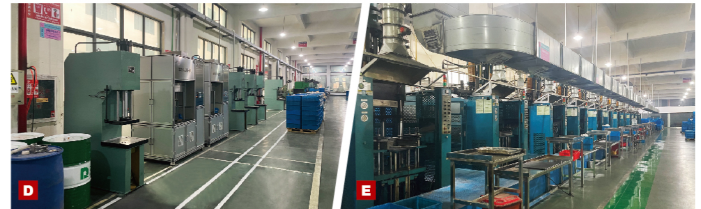
A Metal surface automatic phosphating line B Shot blasting cleaning line C Automatic spraying line D Hydraulic mounting vacuum dry filling production line E Rubber-injection molding vulcanizing machine
