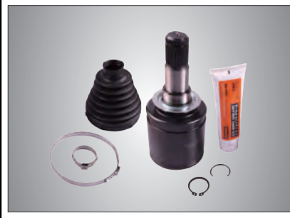
DRIVE SHAFT BOOT ( MATERIAL: RUBBER )
