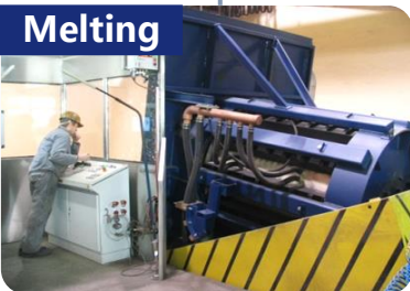
埃博普-6吨中频无芯感应电炉 ABP-6 tons medium frequency coreless induction furnace
