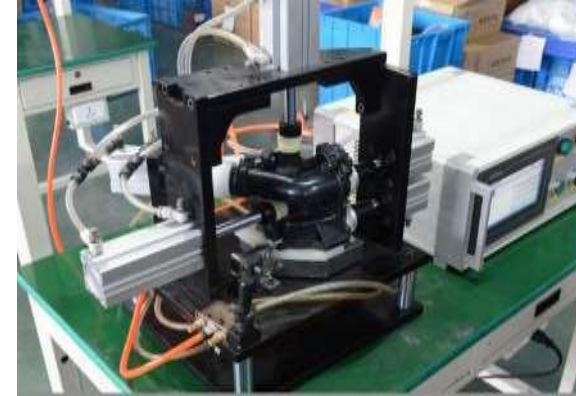
Air Tightness Test
