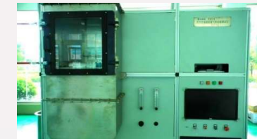
Cabin filter (carbon media) deodorization performance
