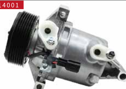
CR08B Nissan Versa Micra 2012-2018 带轮槽数/No. of Grooves: PV7 皮带轮直径/Pulley Diameter: 100mm 926006053R 额定电压/Rated Voltage: 12V 926001HC2D 制冷剂/Refrigerant: R134a 926001KA3B
