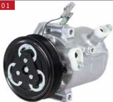
VCR08 Mitsubishi Attrage 带轮槽数/No. of Grooves: PV6 皮带轮直径/Pulley Diameter: 115mm 7813A385 额定电压/Rated Voltage: 12V 7813A526 制冷剂/Refrigerant: R134a
