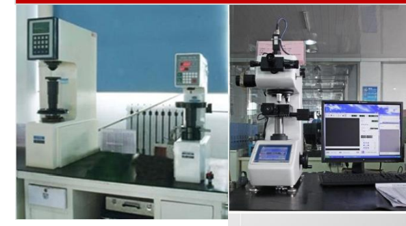
Electronic Rockwell hardness tester, Electronic Brinell Hardness Tester, Electronic dimensional hardness tester
