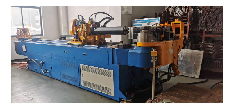
We can bend sway bars with big diameter till 50mm
