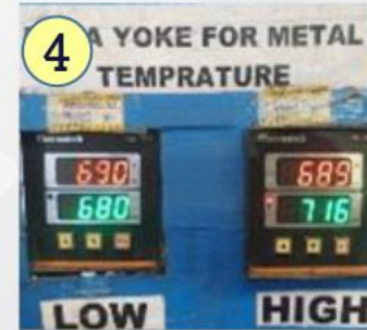
4 Poka Yoke for holding Furnace Temp. < 680~720 Degree >
