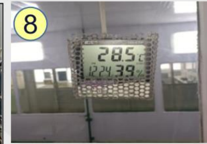
Humidity & Temp Control <Temp spec: 25±3°C Humidity: 55-75 % RH>
