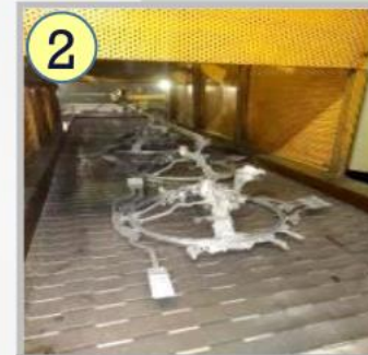
2 Conveyor with Air Cooling < Right Temperature part for Trimming >
