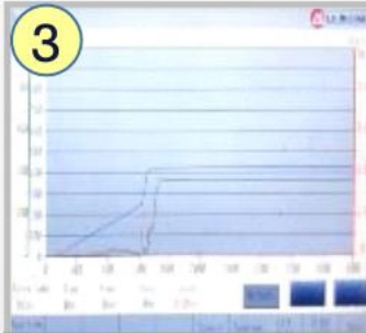
3 Online Process Parameter Record & Control < M/c alarm if out of range >
