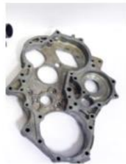
Timing Gear Case
