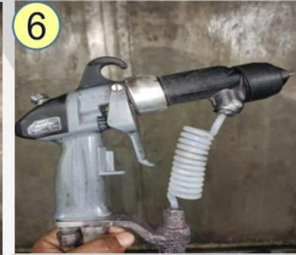
Electrostatic Guns <Effective Paint Coverage>
