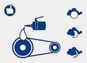
Check the metals and bearings of pulleys for periodic oiling.
