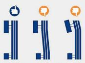
Check the pulley for alignment. Incorrect alignment may result in a shorter belt life.
