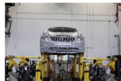
Vehicle Axle Coupling Road Simulation Test
