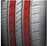
Streamlined staggered transverse groove, with scattered fine pattern sipes.
