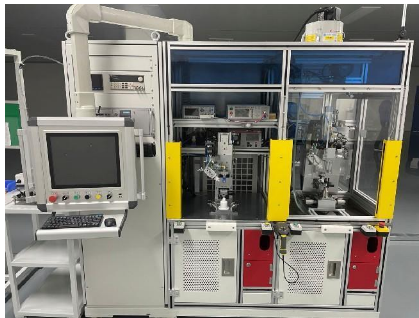
EOL test bench (Detect resistance/inductance/leakage/dynamic flow/static flow )
