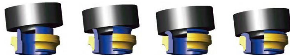
卷边结构形成过程 The forming process of the flanged structure
