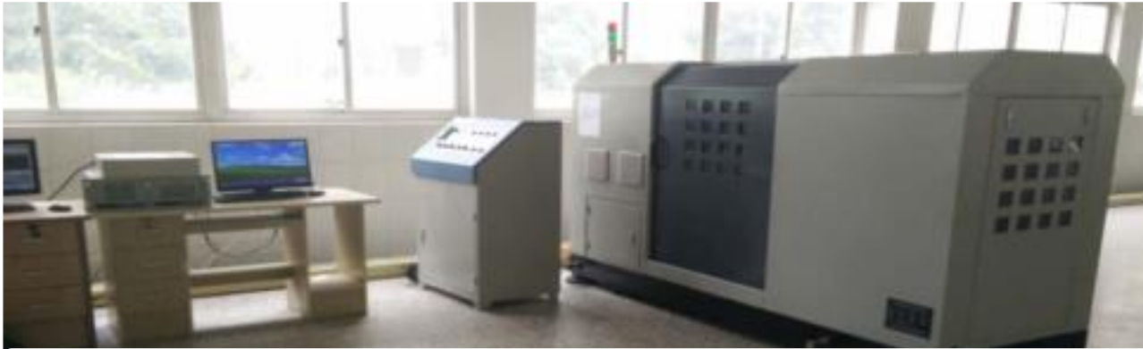
Flange rotating fatigue test machine
