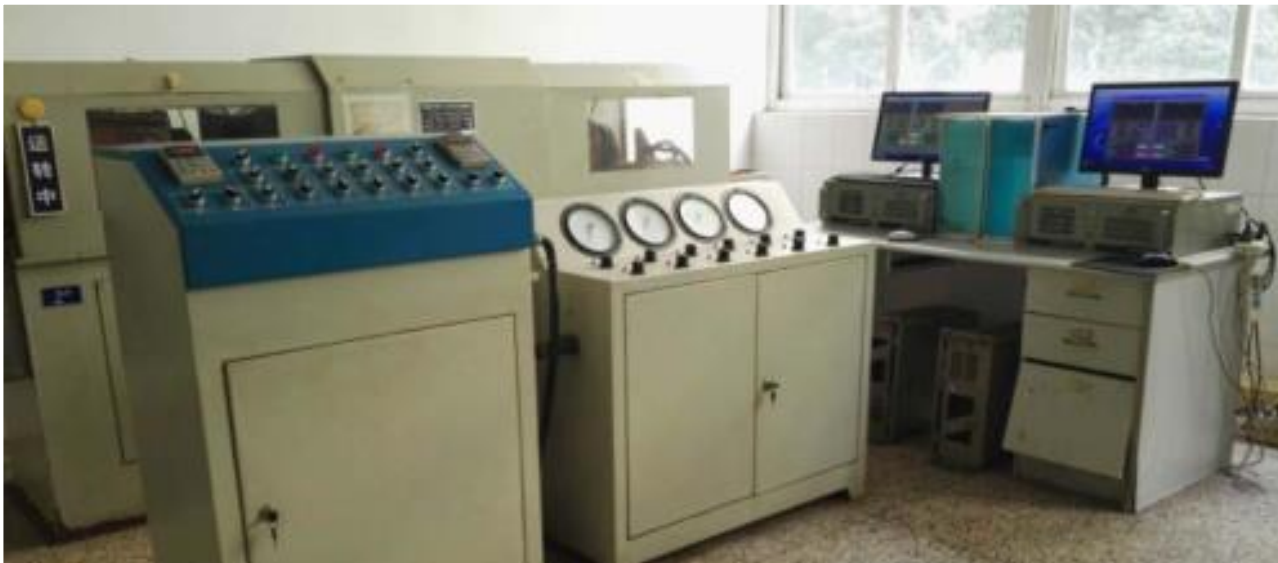
Wheel bearing / unit mud/salt water spray durability test machine
