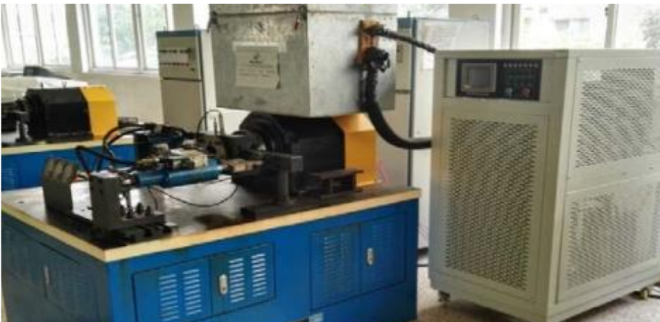
Wheel bearing/unit simulate high/low temperature test machine
