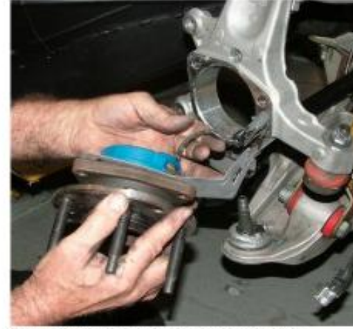
Separate the module from the knuckle, using extreme caution when prying between the two.
