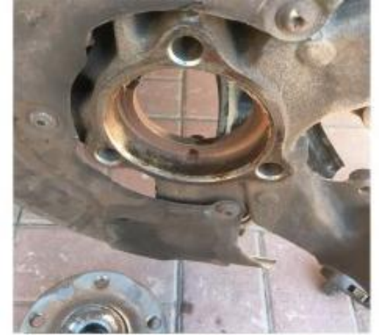
Remove any loose metal from the bearing housing, and inspect the CV shaft for any damage.
