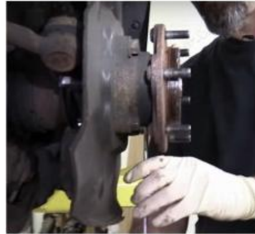
Torque hub mounting bolts to the manufacturer's specifications using the correct torque wrench.
