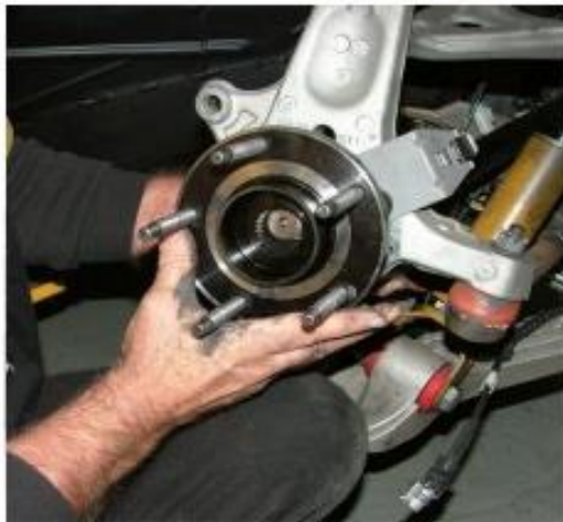
Align the new module onto the CV shaft and in to the knuckle.
