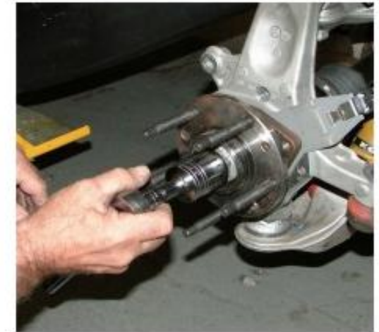
Torque axle nuts to manufacturer's specifications (do not use an impact wrench).
