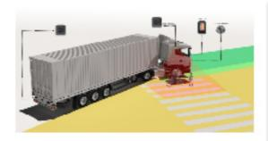
BSIS – Blind Spot Info System for the Detection of Bicycles met European guidelines according to UN ECE R151.
