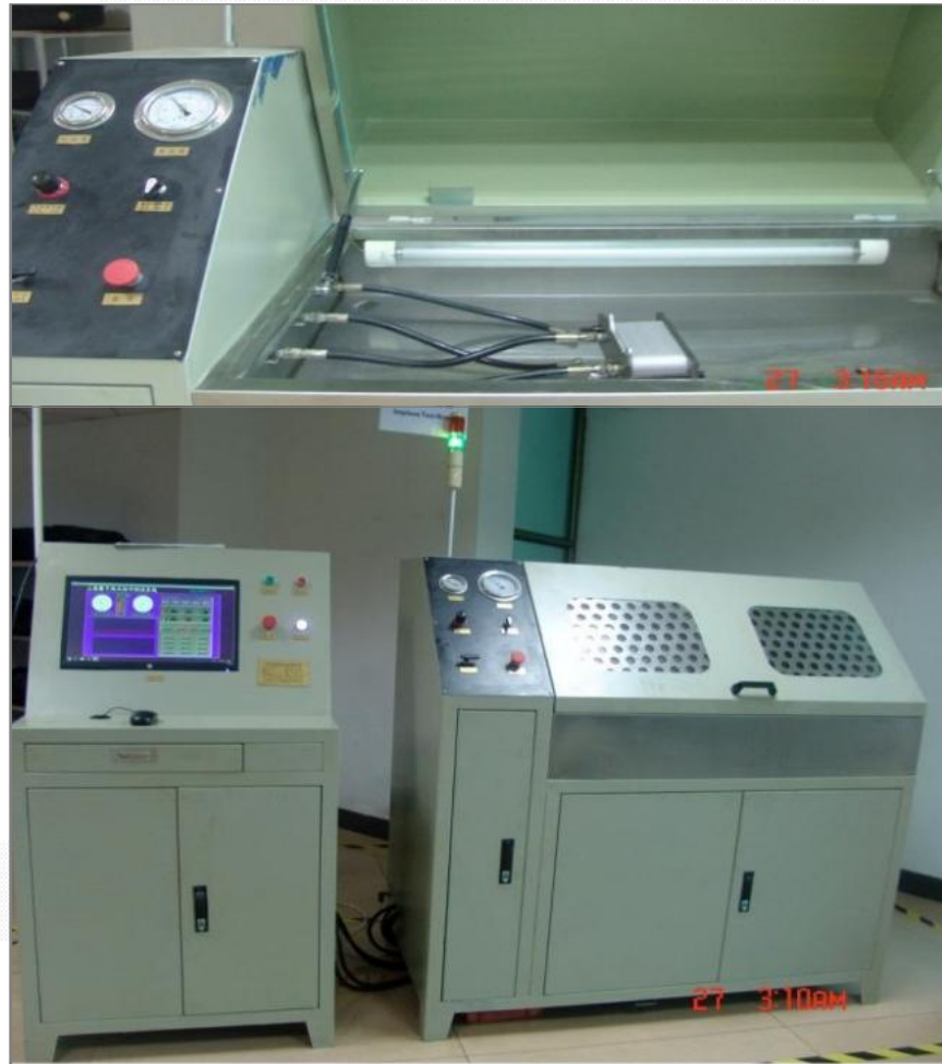
Oil Cooler impulse(life span) testing
