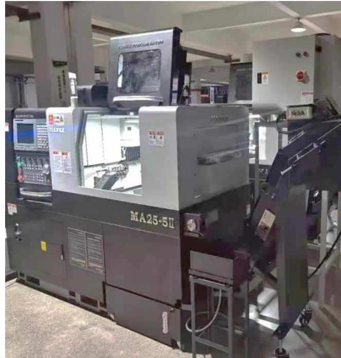
双主轴走心机, 融合机床上下料系统, 轴类, 螺丝, 球头等零件全自动生产 Double spindle precise digital-controlled machine, integrated loading and unloading raw material system, automatic production of shaft parts, ball joint, banjo
