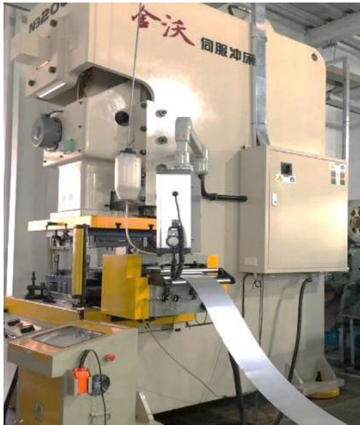
Automatic continuous transfer punching -progressive blanking die
