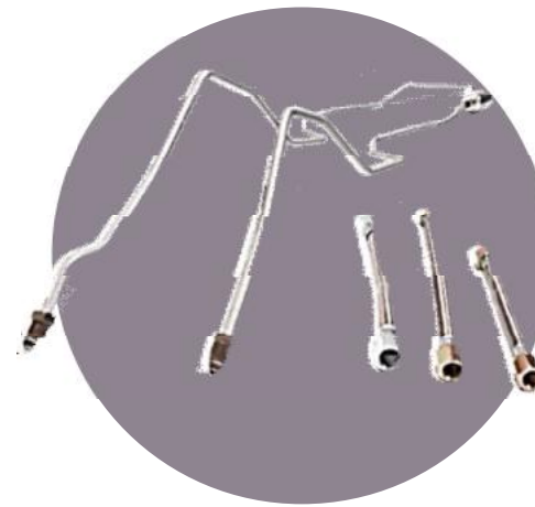
Brake line Material: stainless steel + stainless braided
