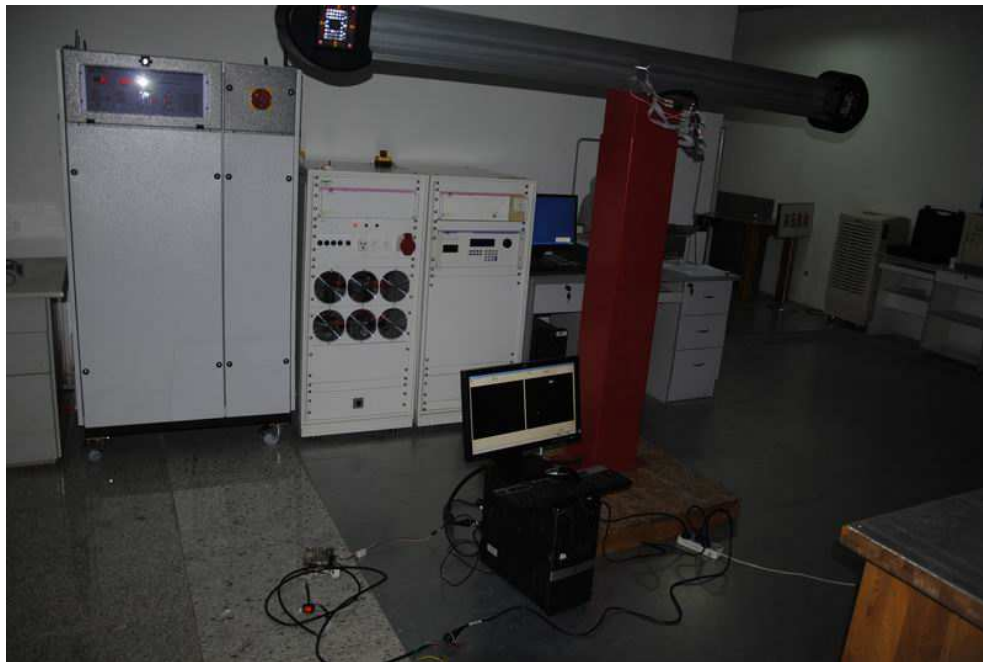
Photograph 2: Set-up for measurement of disturbance voltage
