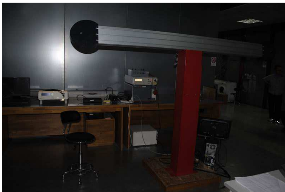
Photograph 6: Set-up for electrical fast transients, surge, voltage dips and interruption
