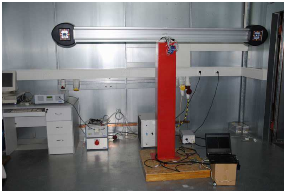
Photograph 2: Set-up for measurement of disturbance voltage
