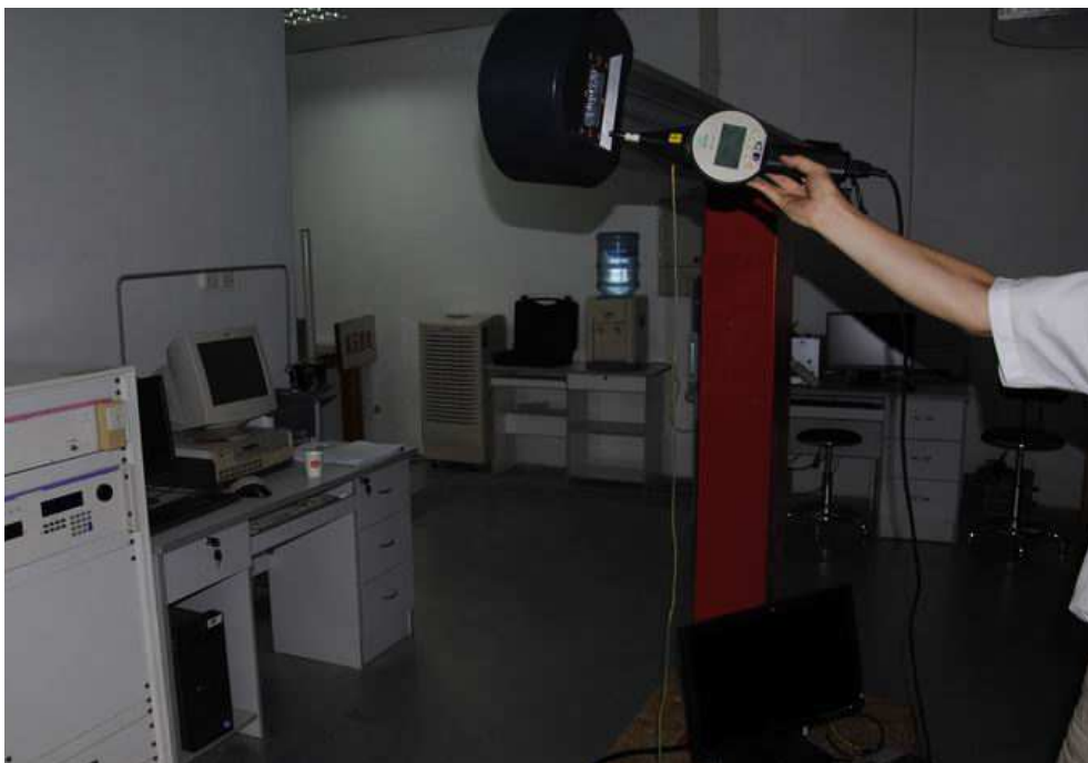
Photograph 4: Set-up for ESD
