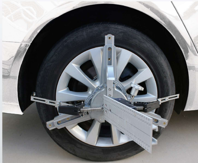
Self centering three finger fixture and laser target ruler
