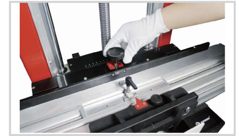
Move the beam left and right by adjusting the knob left and right
