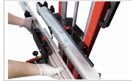
The cross beam is dismantled and mounted for easy storage
