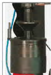
Adopt pneumatic locking device, operating easily and conveniently
