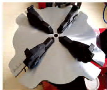
28" turning table, Clamping jaw can be adjusted to 30"
