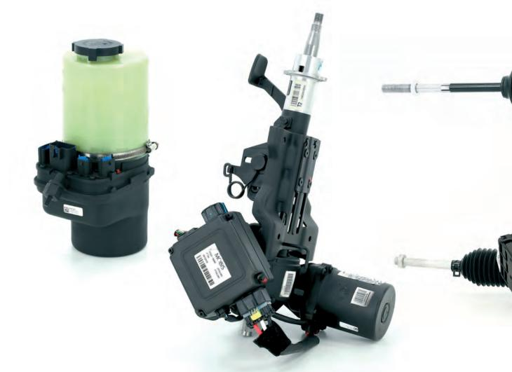
All steering components undergo rigorous testing prior to shipment to ensure that that the shipped product is functional and, above all, safe. We send steering racks equipped with new rods and rack boots so the product is ready for installation in the vehicle.
