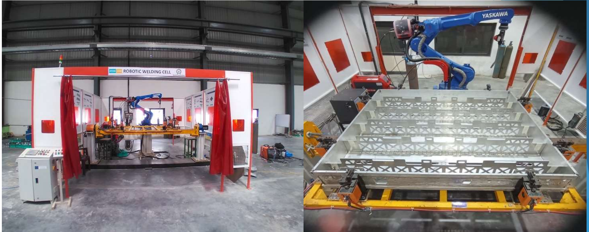
Aluminium MIG welding robotic setup with Yaskawa Robot and Fronius Welding machine
