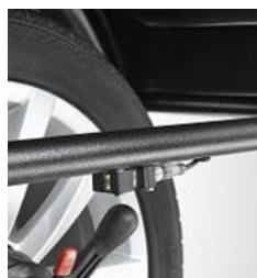
Sonar system for automatic input of wheel width
