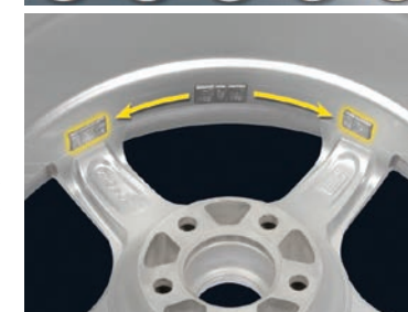
SPLIT (Hidden Weight) program to divide counterweights behind spokes of alloy rims.
