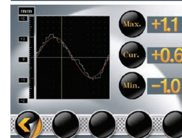
Eccentricity measuring system (1st harmonic and peak to peak) through Ultrasonic sensor.
