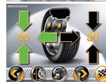
ALU-S function with "intelligent" gauge (automatic input of diameter and distance rim/machine) for correction on the wheel. Axial weight position indication by arrows.
