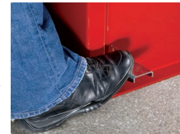
Footbrake to ease locking and unlocking wheels on adaptors as well as for counterweight fitting.
