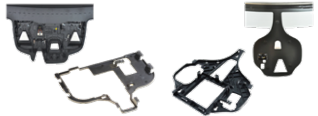
Assembly plate bonded to the windscreen.
