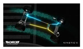
High wheel articulation and better wheel load distribution give the car more stability and much higher traction on rough terrain. The system's ability to completely disconnect the roll stiffness of the system allows the wheels to travel independently to maintain contact with the ground even in the most extreme conditions. Overcoming challenging obstacles is all in a day's work for this suspension system.
