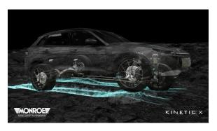
Kinetic X, in fact, adds pitch control to the existing damping and roll control capabilities of the successful Kinetic H2 system. The Kinetic H2 system was the first suspension system introduced by Monroe, offering roll control, and eliminating the need for a mechanical roll bar. By adding pitch control, the Kinetic X system further raises handling, safety and ride experience to levels never achieved before- by brining pitch movements of the vehicle to a standstill.
