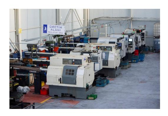
14 x C axis CNC Lathe
