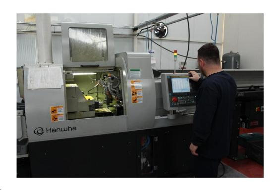
There are 3 CNC Sliding Automats, which are up to 8 axes. The processable material capacity is between Ø3 and Ø26 mm.
