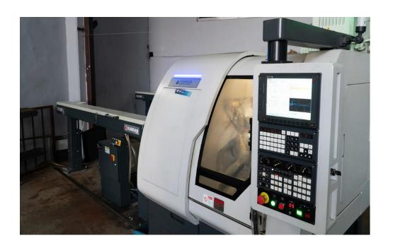
11 CNC turning lathes up to 4 axes, materials between Ø3 and Ø 32 can be processed.
