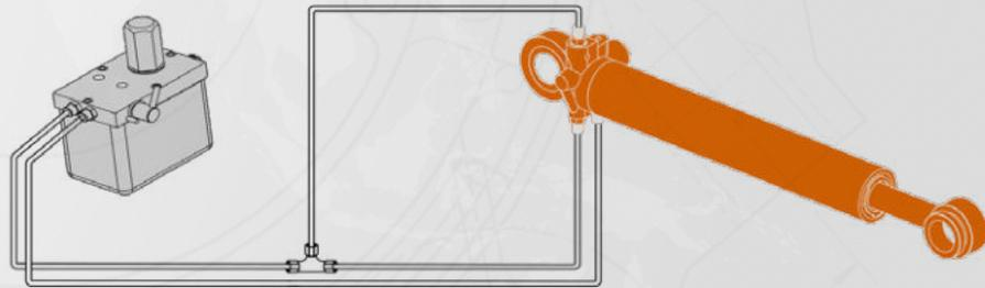
The primary function of the Cabin Tilting Cylinder is to generate hydraulic force that enables the controlled tilting motion of the driver's cabin. It operates by utilizing hydraulic pressure to extend and retract a piston, which in turn moves the tilting mechanism. The cylinder is usually integrated with a locking system that securely holds the cabin in position during maintenance operations.
