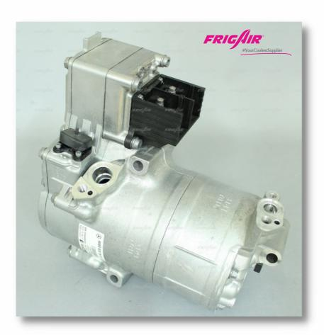
Many high-voltage compressor models have two connectors in the unit. The larger connector is used for the high-voltage connection to the vehicle's battery. For safety reasons, both the connector and the wiring to the battery are brightly colored in orange to indicate high voltage.
